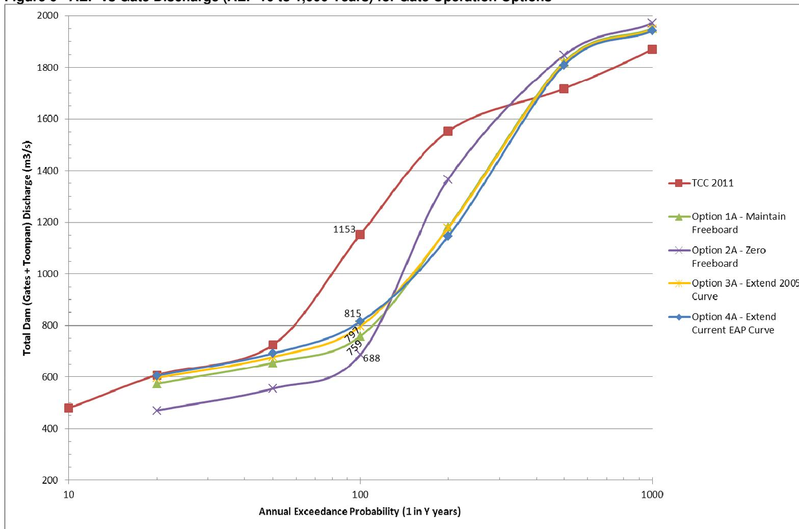
Figure 7 - Peak Flood Discharge Comparison (Total Dam Outflows)
