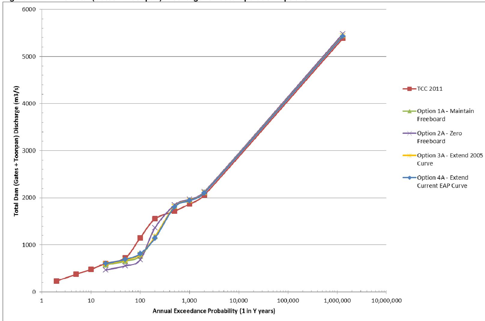
Figure 6 - AEP vs Gate Discharge (AEP 10 to 1,000 Years) for Gate Operation Options
